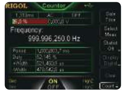
Standard 7 digits/s full function frequency counter with 200MHz bandwidth
