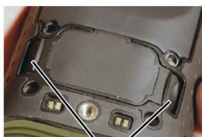
Grasp SD Card door edges and pull
