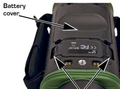
Grasp SD card door edges and pull
