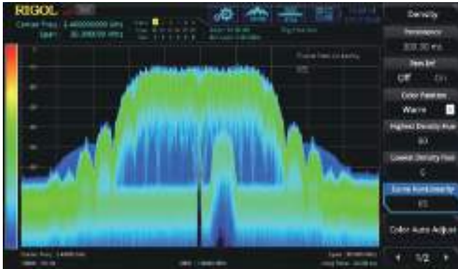
With the Density spectrum, you can find out the exceptional signals hidden behind the high-level signals, and capture them accurately with the FMT.
